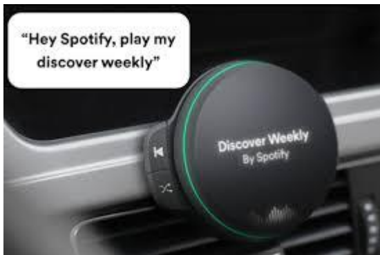
Car Thing connects to 12-volt outlet and uses the phone connection. Responds to voice commands.
